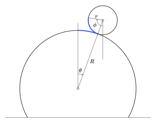
We let  $\theta$  denote the angle travelled by the hoop with respect to the surface. Similarly,  $\phi$  corresponds to the angle between a vertical line through the hoop, and the original position of the hoop. We seek to find  $\theta$  at the point where the hoop stops rolling, and falls from the cylinder.
