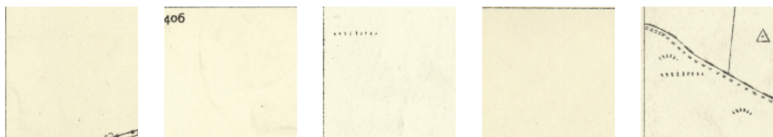
Figure 3.10: Examples of patches which have border pixels. Our filtering algorithm will remove the first 4 of these patches, since most of the information that they contain is in the border pixels. However, the last patch will be preserved in the dataset, since it does hold informative value.
